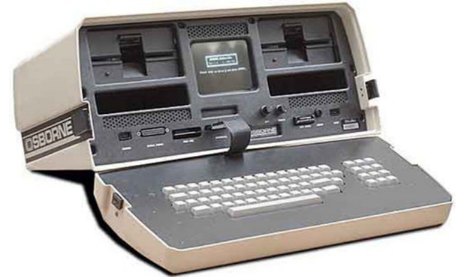
Osborne 1, the first “portable” computer – only 10 kilos.
