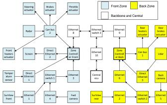
Fig. 4. Zone-based implementation of the hardware resources.
