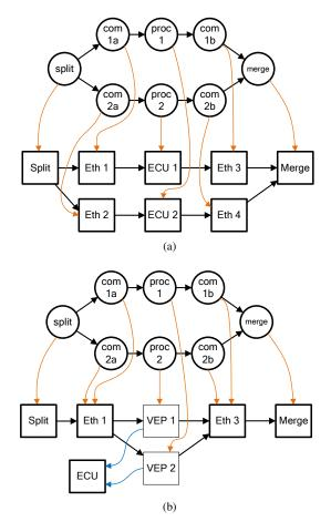
Fig. 1. Phylscal separation (a) and virtualization of resource ECU (b) for independence of redundant application nodes. Black arrows represent samelayer logical interconnections, orange arrows are inter-layer mapping edges, blue arrows link the VEPs to the original resource in the resource layer.
