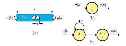
Fig. 10 Example of a conveyor belt and its dataflow linear model
