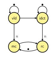
Fig. 1 A dataflow model of an H.263 decoder
