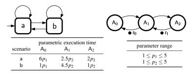
Fig. 13 An SADF with parametric actor firing delays
