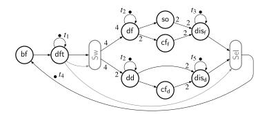
Fig. 22 The merged execution graph, the switch and select actors are indicated in grey.
