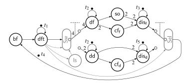
Fig. 23 The merged execution graph with implementation details, the *switch/select* and *load sched-ule* (ls) actors for a one-processor mapping are indicated in grey. The swapping of FIFO channels is indicated with the electrical symbol for a switch, also in grey. Note that this is not a valid dataflow graph.
