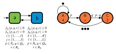
Fig. 11 Example of a parameterized SADF.
