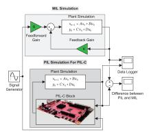
Fig. 7. Block diagram for PIL-C simulation created in Simulink Environment.
