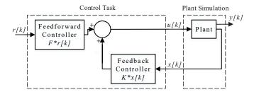
Fig. 2. 2-DOF feedback-feedforward tracking control structure.
