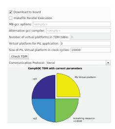
Fig. 6. The created menu in the tool-chain which enables the designer to define TDM variables as well as communication channel for the simulation.
