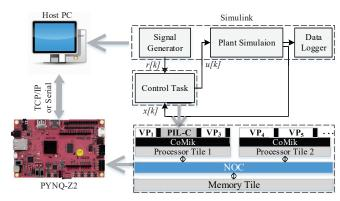
Fig. 4. PIL-C configuration. The embedded platform is implemented on a PYNQ-Z2 FPGA board. The host PC which runs Simulink communicate with the board through TCP/IP or serial connection sending r[k] and x[k], and receiving the resulted u[k].
