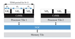
Fig. 1. Predictable embedded platform under consideration.
