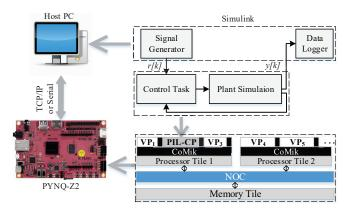
Fig. 5. PIL-CP configuration. Both control task and plant simulation are simulated on the platform. The host PC which runs Simulink communicate with the board through TCP/IP or serial connection sending r[k], and receiving the resulted y[k].
