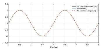
Fig. 8. PIL simulation output for PIL-C configuration. The MIL and PIL results are identical in this configuration.
