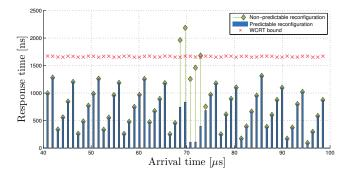
Figure 12: Response times with and without predictable reconfiguration.
