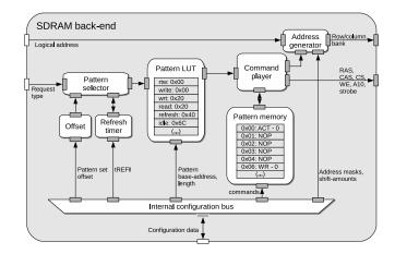
Figure 9: Reconfigurable SDRAM back-end.
