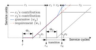
Figure 7: Example of the latency-rate guarantees during reconfiguration.
