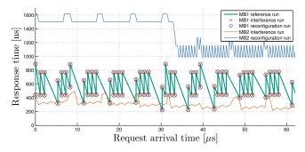
Figure 14: Request latencies using composable patterns.
