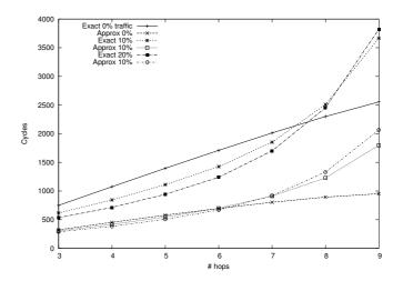
Figure 4: Allocation time vs. path length using 0%, 10% and 20% background traffic.
