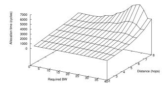
Figure 5: Allocation time vs. path length and requested bandwidth, Exact method, 10% background traffic.
