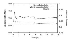
Fig. 8. Net bandwidth plotted over time for a DDR2-400 memory with and without worst-case switches.
