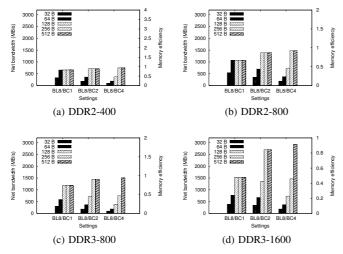
Fig. 7. Bound on net bandwidth for different memories and request sizes.
