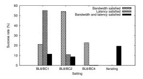
Fig. 9. The percentage of use-cases with bandwidth and latency requirements satisfied using pattern generators with fixed and iterating burst counts.
