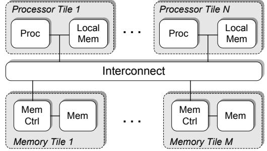
Fig. 1. General tiled-architecture template
