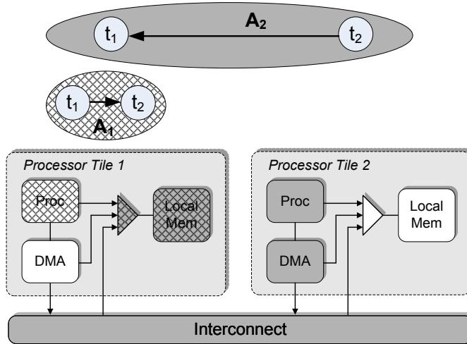
Fig. 4. Example: two application sharing MPSOC resources
