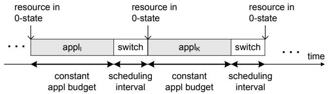
Fig. 2. Composability via zero interference
