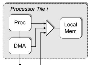
Fig. 3. Basic processor tile with DMA (logical view)
