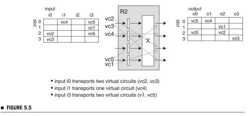
Virtual circuit switching with a single buffer per link and TDM.
