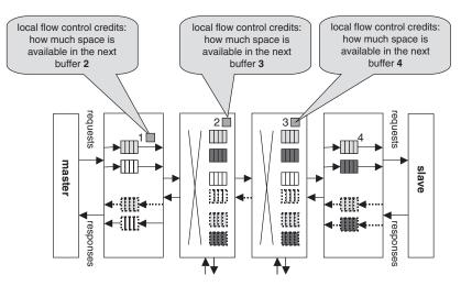
• master-slave uses light-shaded solid and dashed circuits for requests and responses, resp.
