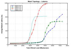
Figure 9. Average Network Latency versus Total offered load for different mesh instances.
