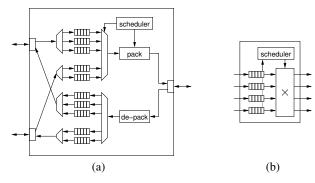
Figure 2. Example of NI architecture (a) and router architecture (b).
