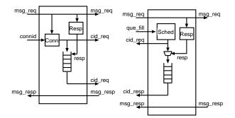
Figure 3. Narrowcast shell Figure 4. Multi-connection shell
