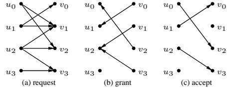
Figure 3. The three stages of a schedule iteration.
