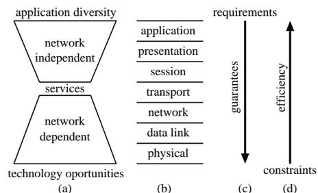
**Figure 1.** Network services (a) hide the interconnect details and allow reusable components to be build on top of them, (b) are build using a layered approach (c) are driven by the application requirements, and (d) their efficiency relies on technology and network organization.
