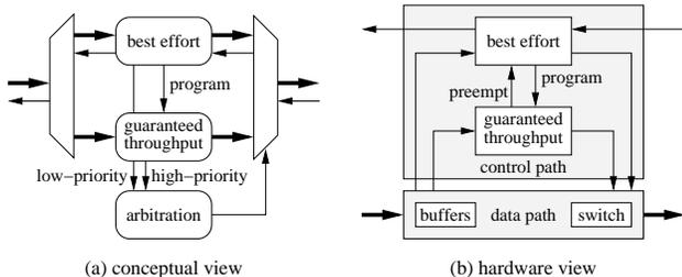
Figure 4. Two views of the combined GT-BE router.
