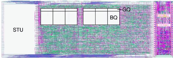
Figure 5. Lay-out of a combined GT-BE router.
